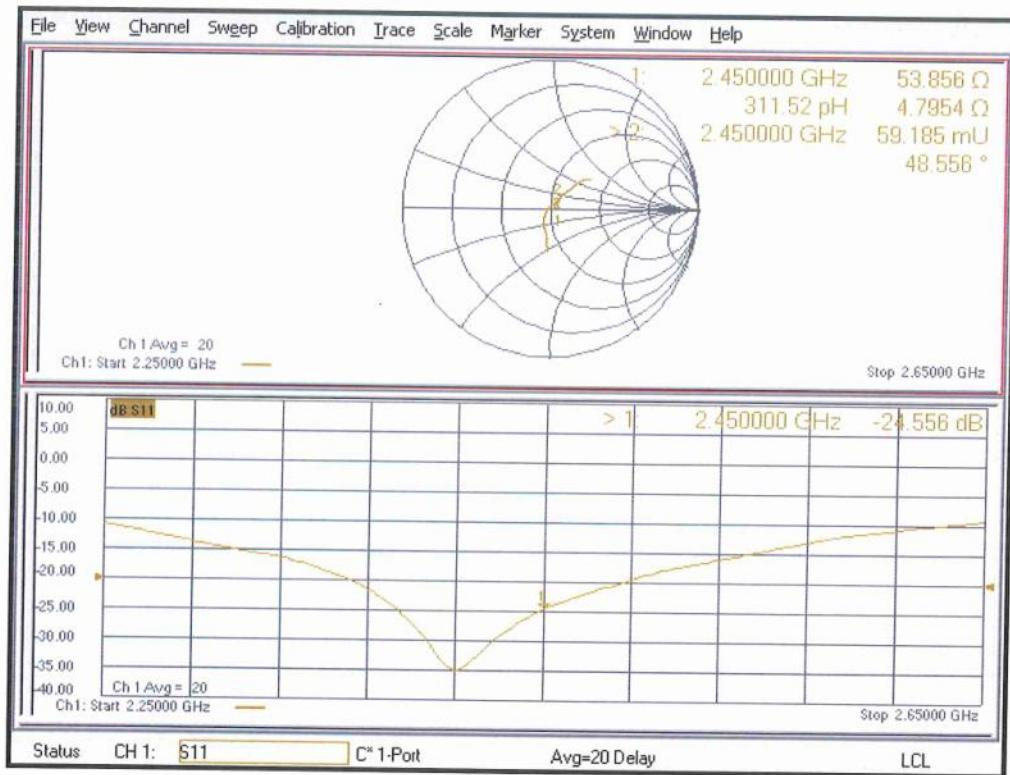
**D2450V2 - SN:1102 Extended Dipole Calibrations**
