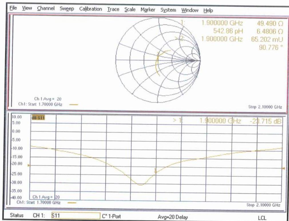
**D1900V2 - SN:5d251 Extended Dipole Calibrations**
