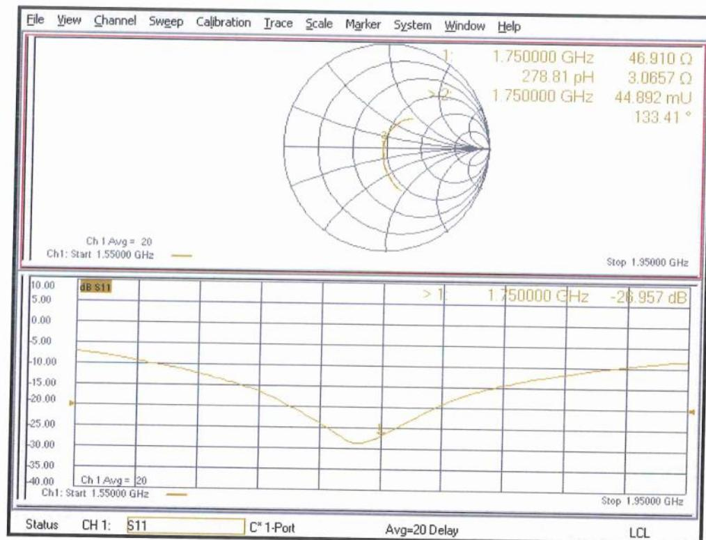
**D1750V2 - SN:1200 Extended Dipole Calibrations**
