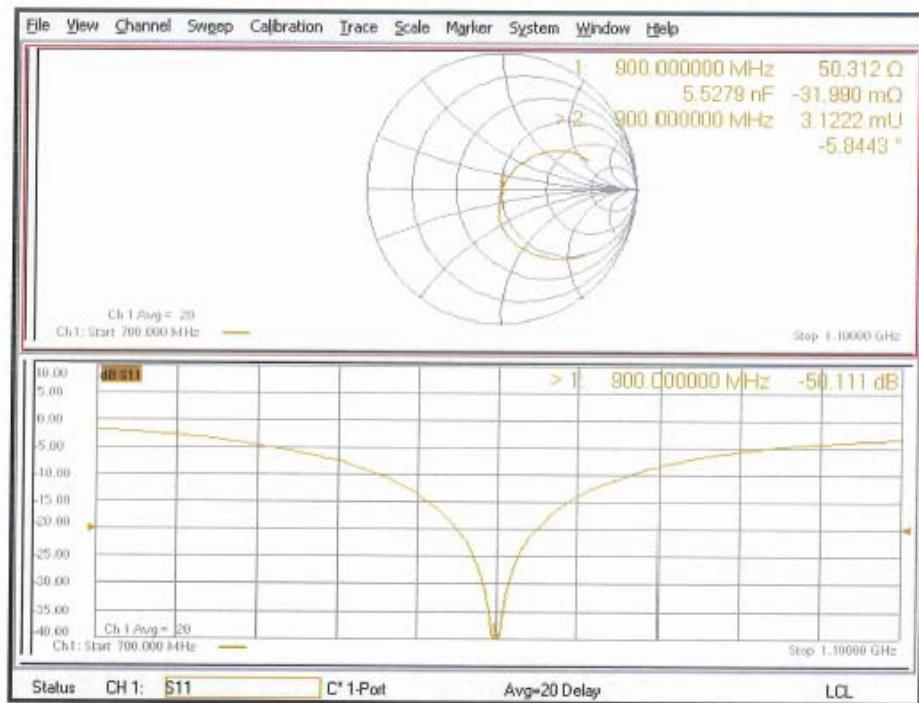
**D900V2 - SN:1d217 Extended Dipole Calibrations**
