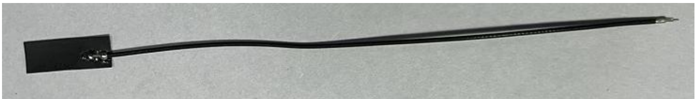
Chart 2 TX2208 Antenna finished (Line length 140+/-2mm)
