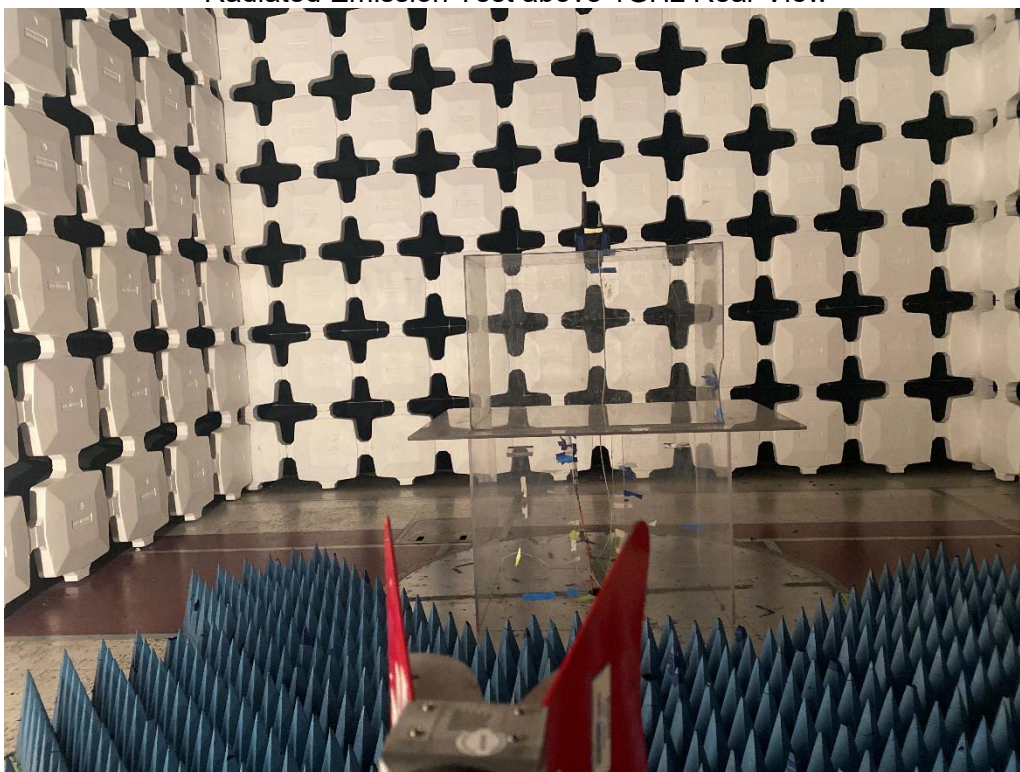
Radiated Emission Test above 1GHz Rear View
