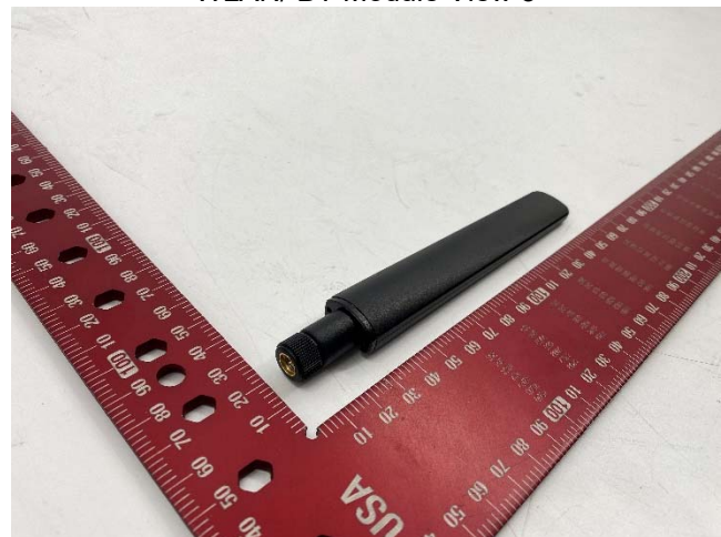
Cellular Antenna View
