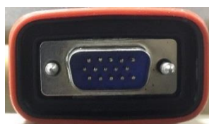
Figure 3.10-3 DB-15 Interface on RRU
