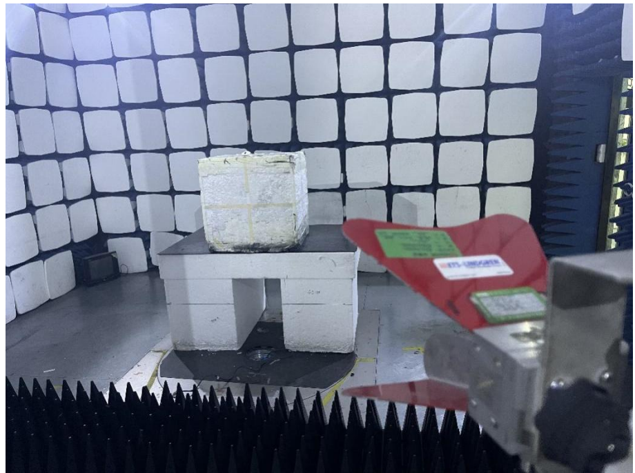
Radiation Emission Test Setup (1GHz to 18GHz)
