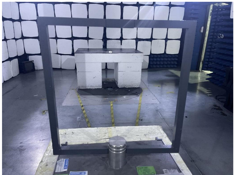
Radiation Emission Test Setup (Below 30MHz)
