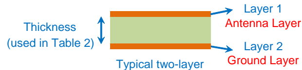
Figure 11. Clarification of PCB Thickness
