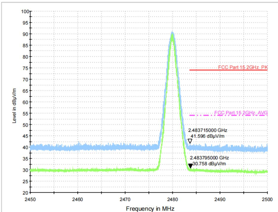
TM4 / Polarization: Horizontal, Vertical / Band: 2.4G / BW: 1 / CH: L
