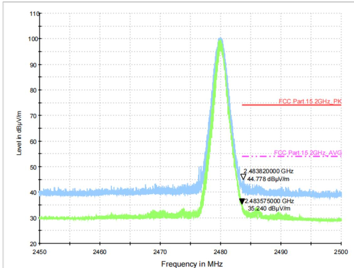
TM3 / Polarization: Horizontal, Vertical / Band: 2.4G / BW: 1 / CH: L
