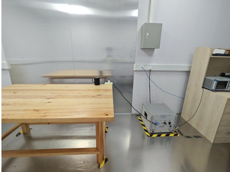
Radiated Spurious Emissions Test Frequency From 30MHz-1GHz
