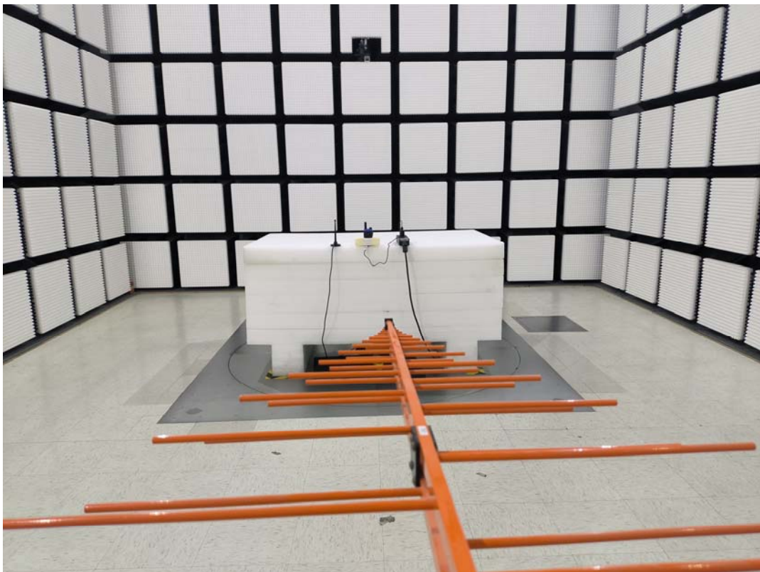
Radiated Emission Below 1GHz Rear View
