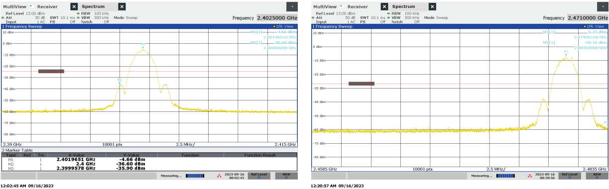
Figure 15: Radiated Emissions at Band Edge, Spectral Diagram, Modes A (2402MHz) and C (2480MHz), 2Mbps
