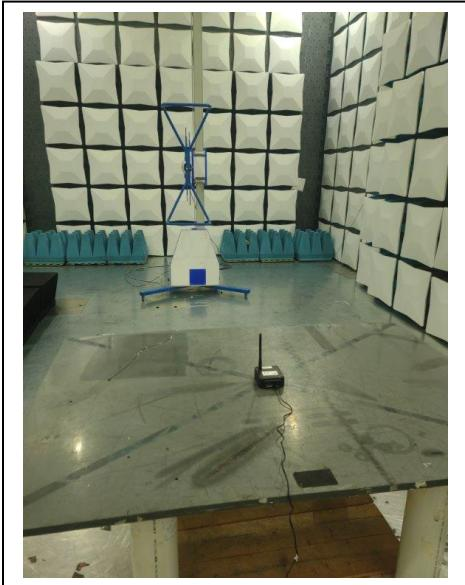
**Radiated Spurious, Less Than 30 MHz**
