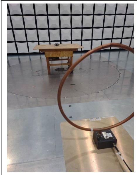
**Radiated Spurious, 1 GHz to 13 GHz**
