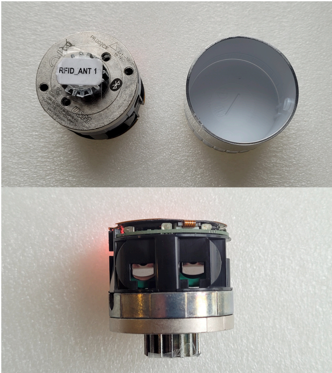
Lock C Internal photos
