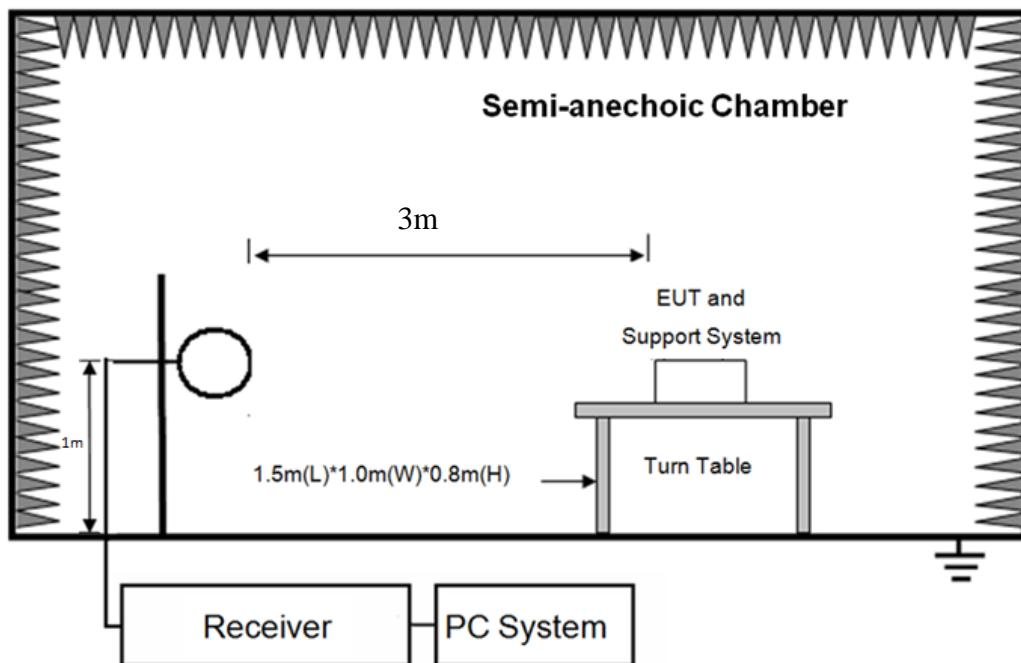
Test Setup Diagram for 30MHz~1GHz
