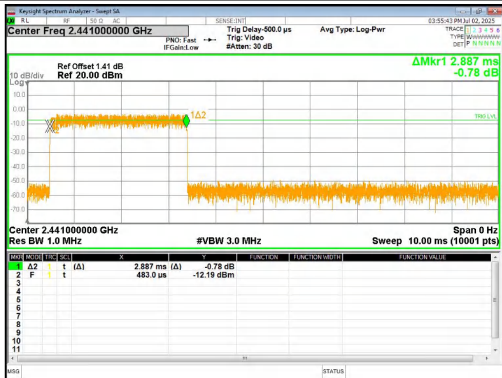
Dwell NVNT 2-DH5 2441MHz Ant1 Accumulated
