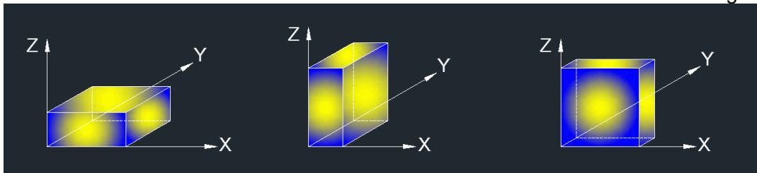
Note: For all radiated test, EUT in each of three orthogonal axis emissions had been tested, but only the worst case (X axis for horizontal and Z axis for vertical) data recorded in the report.
