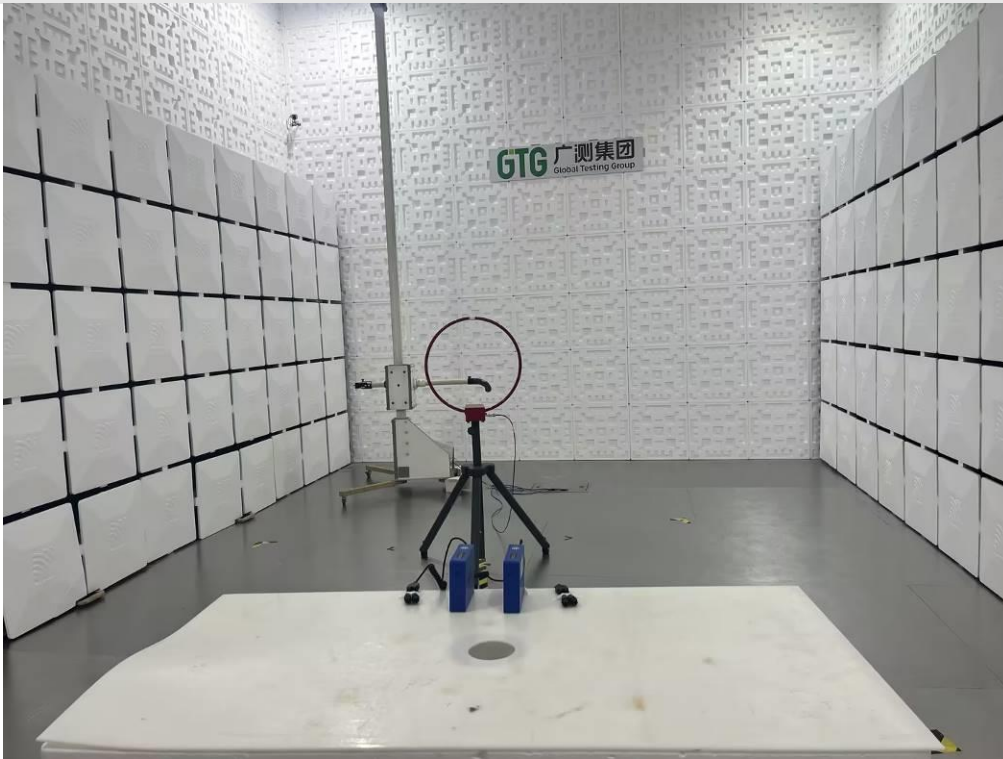
Radiated emissions below 30MHz
