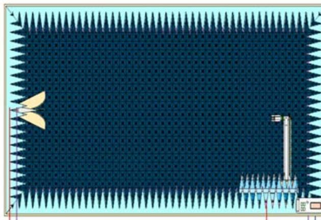
Chamber - MTG 6x3x3(m), 300MHz~6GHz
