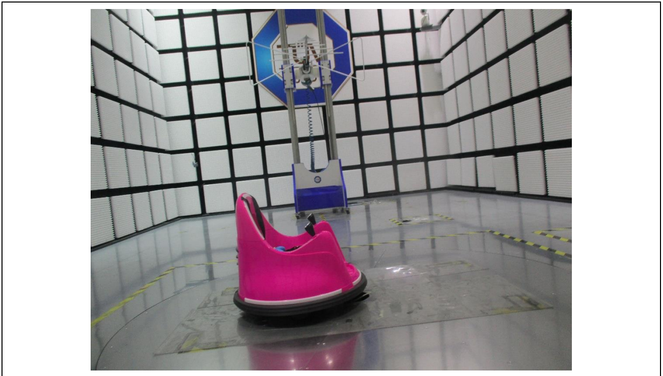
Radiated Emission test (1000MHz to 18000MHz)
