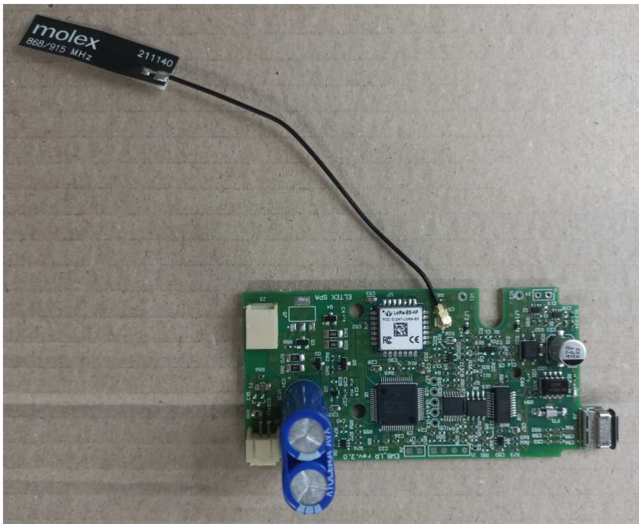
LoRa pcb and connected Molex antenna
