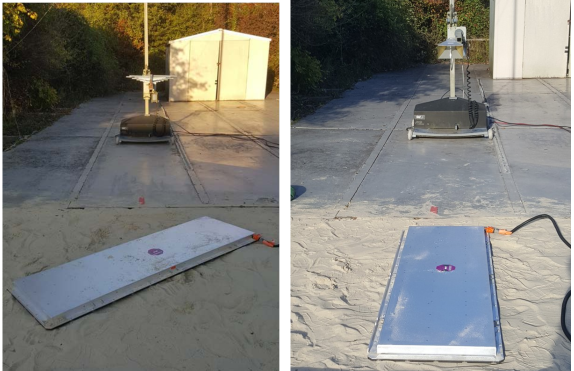
Fig. 3.1 Radiated Emission Test Setup
