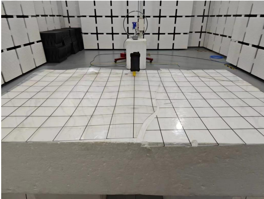
Radiated Spurious Emission Test Setup Photo – 30-1000MHz
