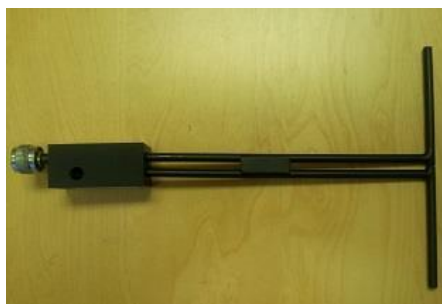
Figure 1 – MVG COMOSAR Validation Dipole
