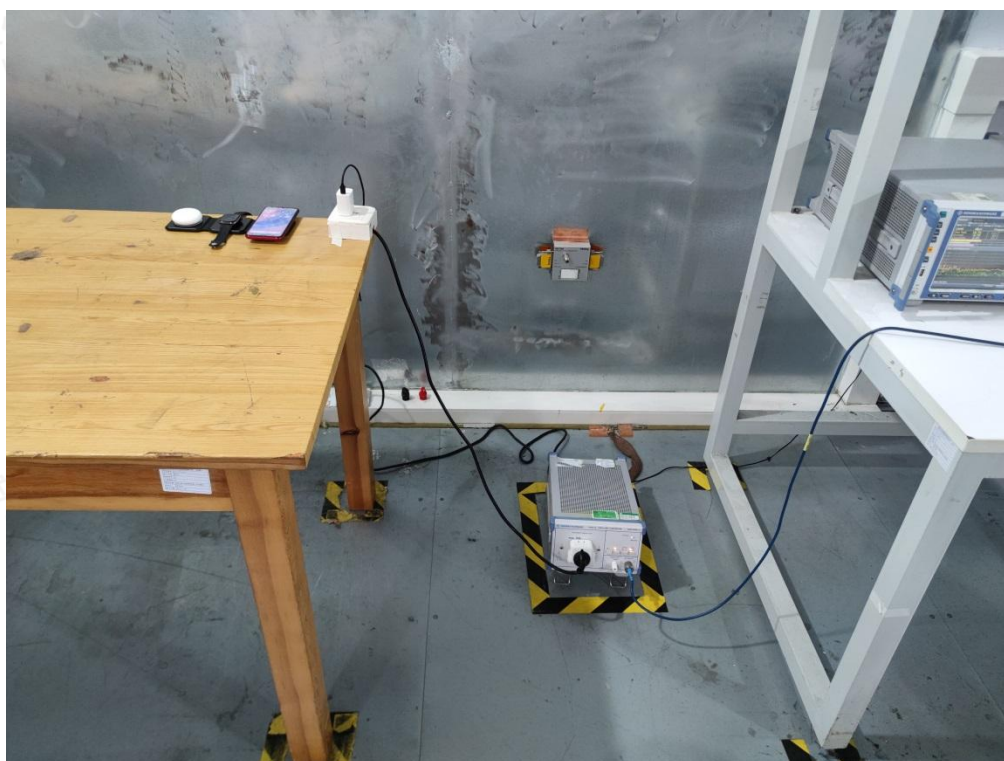
Conducted Emission-AC adapter charge mode
