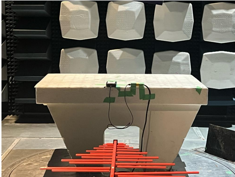
Figure 1: Radiated Emissions (30 MHz-1GHz) performed at the SAC Test Setup
