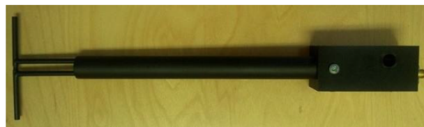
Figure 1 – MVG COMOSAR Validation Dipole
