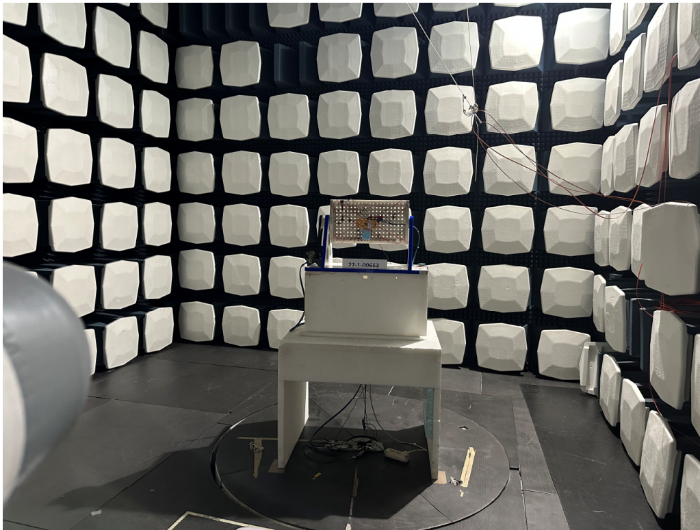
Fig. Mea.: 3 : Measurement in the fully anechoic chamber 1
