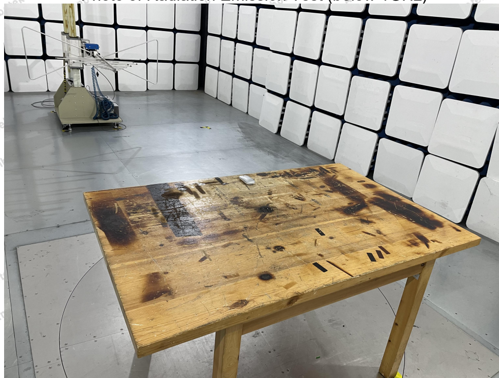
Photo of Radiation Emission Test (below 1GHz)
