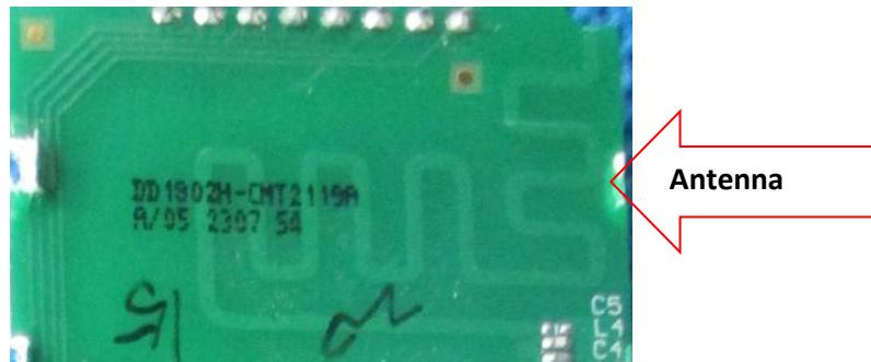
Antenna transmission frequency: 433.92MHz
