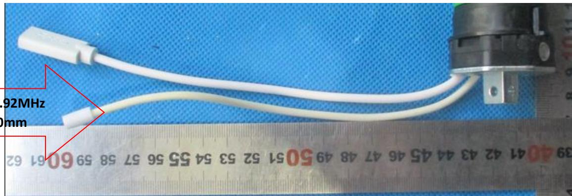
Antenna transmission frequency: 433.92MHz
