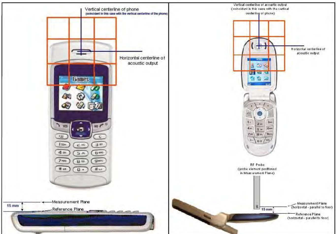
Fig-3.4 EUT Reference and Plane
