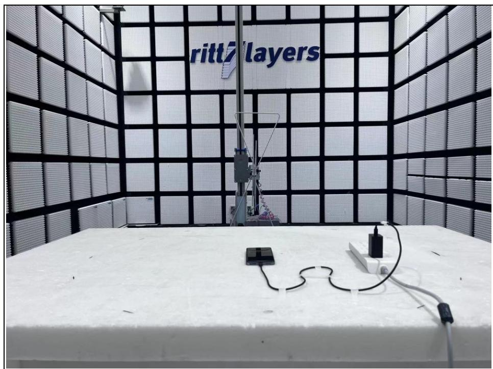
Radiated emission test: Frequency Range< Above 1GHz >
