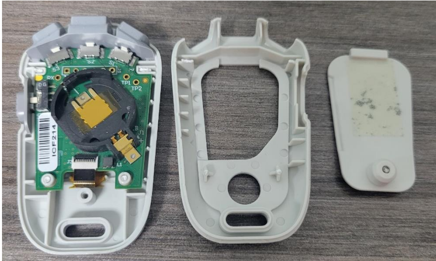
Patient Remote Internal view showing Front Cover with PCBA and buttons, Back Cover, & Battery Door.
