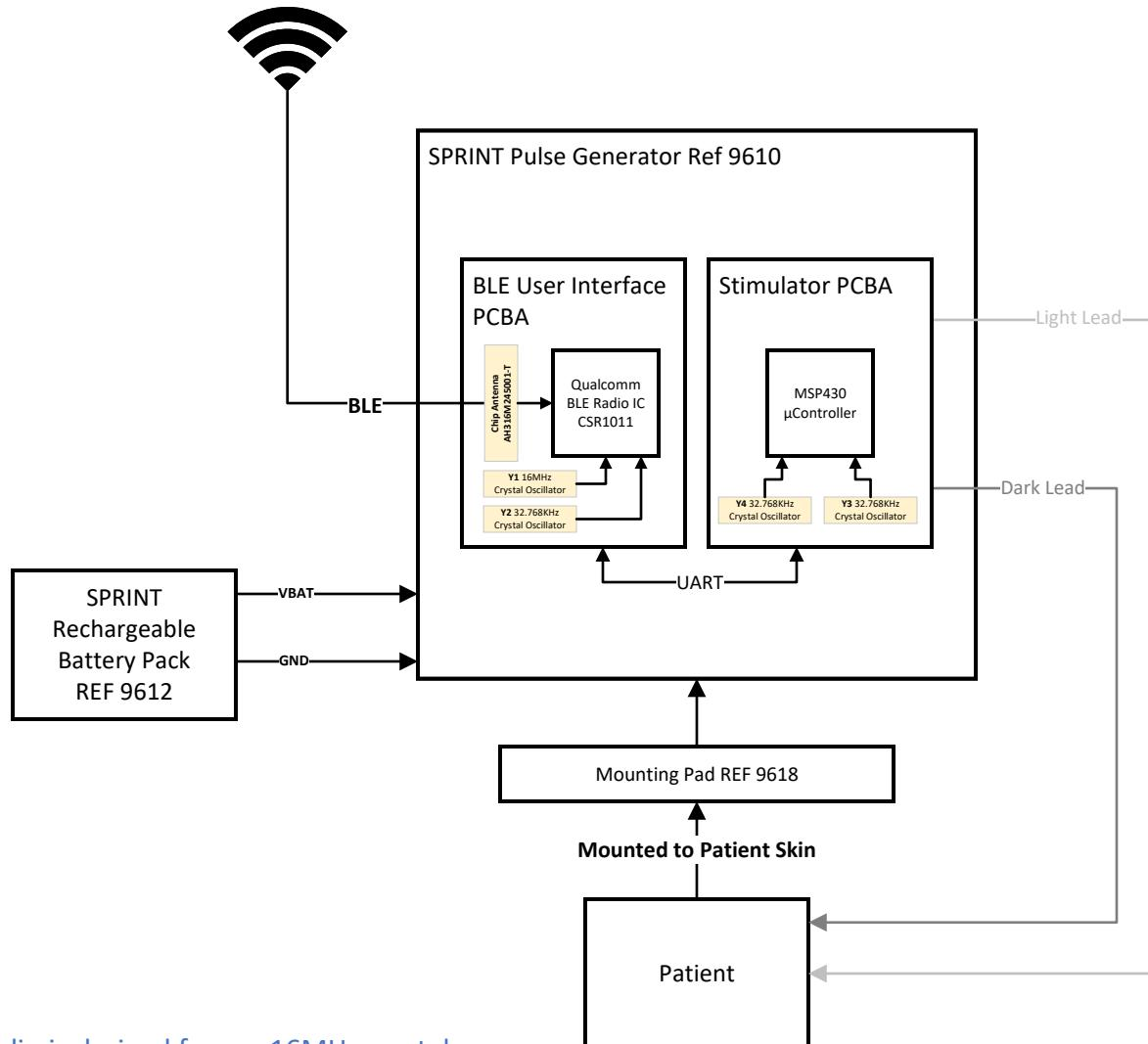
Timing/ clock source for the BLE Radio is derived from a 16MHz crystal oscillator (Y1) that is factory calibrated to 16MHz +/-20Hz (1.25ppm). Y2 is the application clock source for low power/ sleep state.
