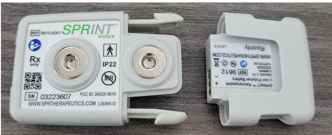
Back View Product Label with FCC ID Number Showing Battery (Ref 9612) and Mounting Pad Connections
