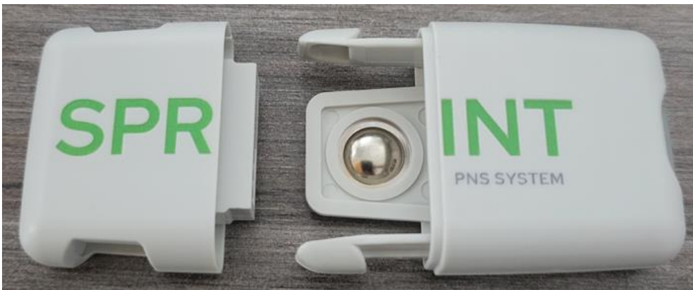
Front View Showing Battery (Ref 9612)
