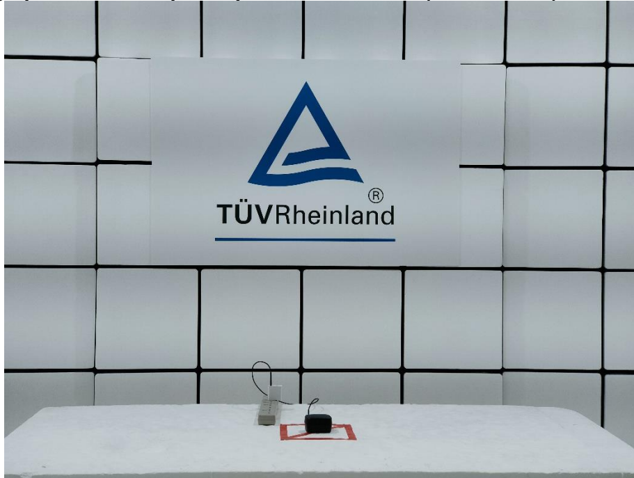
Photograph 8: Test Setup for Spurious Emissions (Back View 1)
