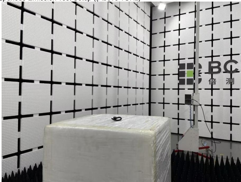
Spurious Emission Test Setup (Between 30MHz – 1GHz)
