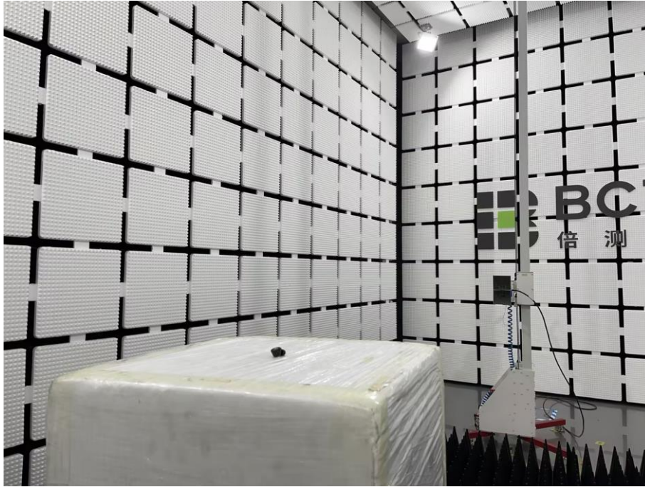
Spurious Emission Test Setup (above 1GHz)
