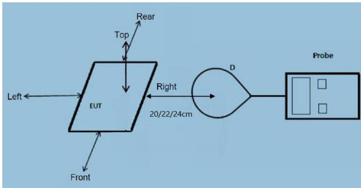
Note: Measurements should be made from all sides and the top of the primary/client pair, with the 20/22/24 cm measured from the center of the probe(s) to the edge of the device
