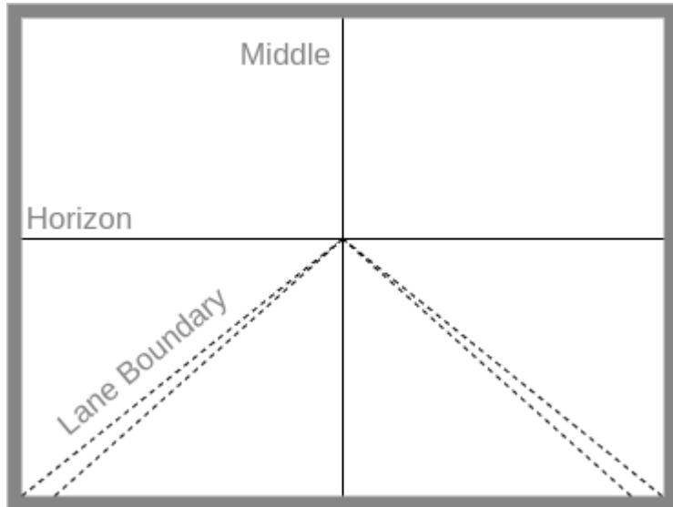
Alignment Guide Lines in Calibration mode. Middle vertical line is the center of the bumper location. Horizontal guide line is for alignment of the horizon.
