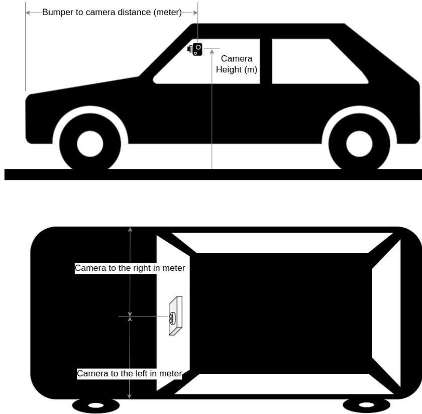
Camera location. Please note that the right camera is the ADAS camera. The distances are measured from the center of the ADAS camera to the boundary.
