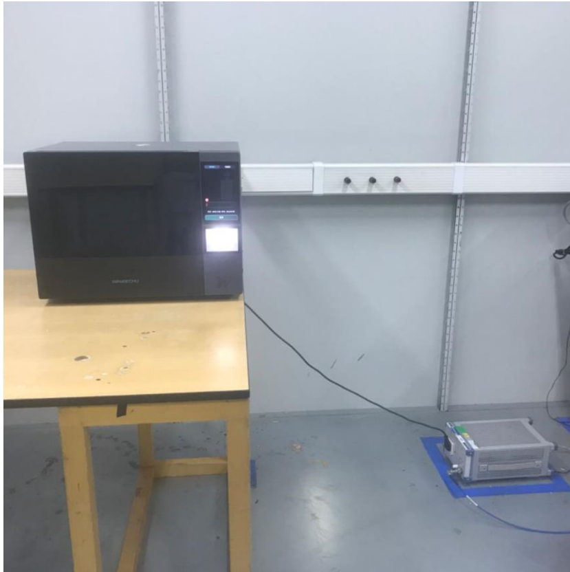
AC Conducted Emission Test Setup -Front
