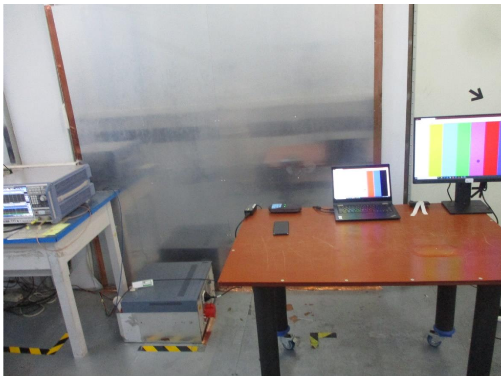
Photograph 4: Set-up photo for Conducted Emission on AC Mains
