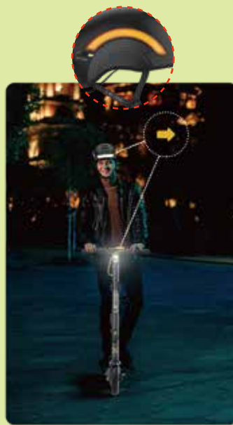
THE HELMET RIGHT LIGHT FLASHES AT RIGHT TURNING.
