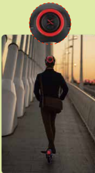
THE BRAKE LIGHT FLASHES AT BRAKING.
