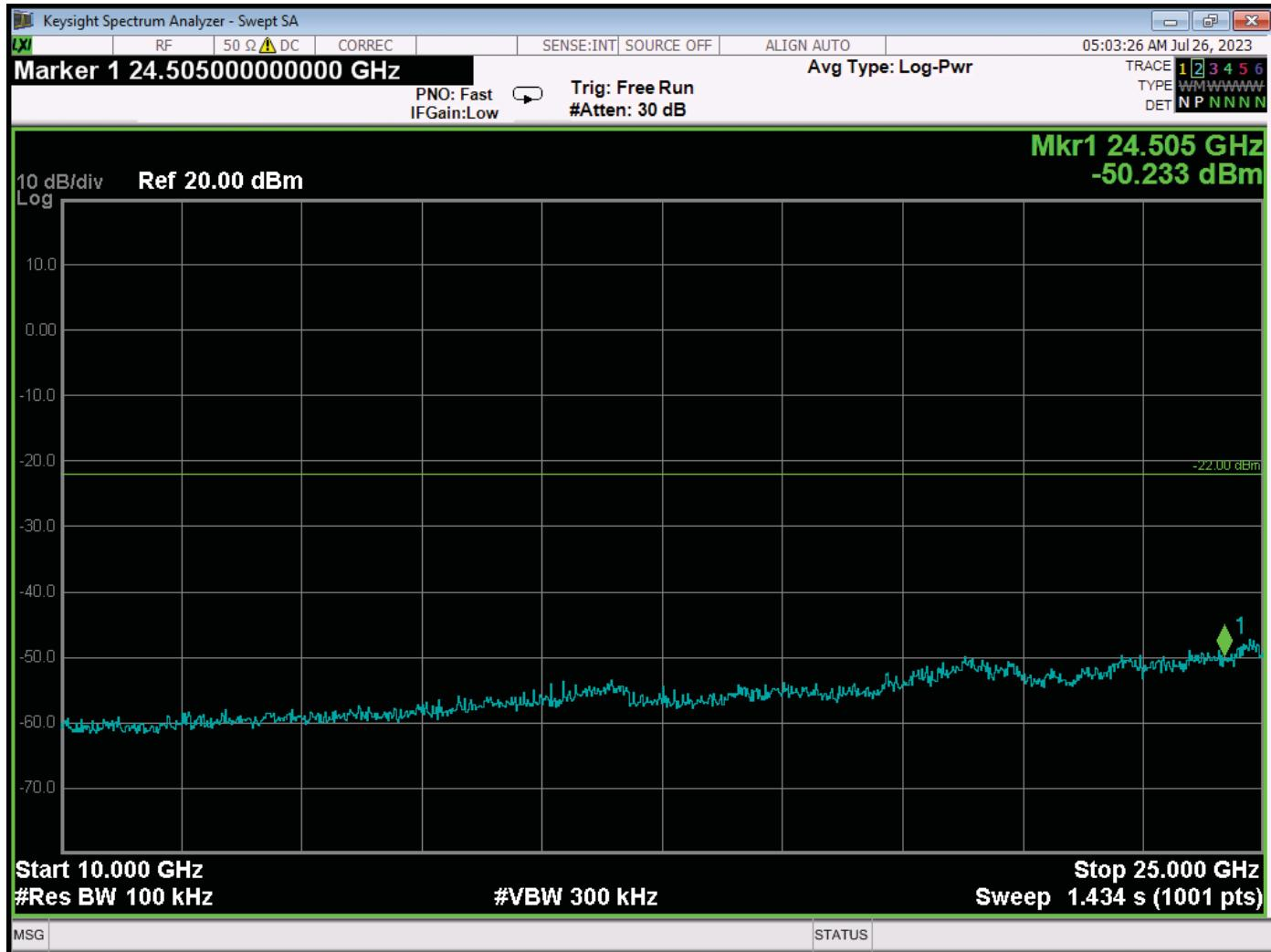
RF Antenna Conducted Test – High Channel – 10 GHz to 25 GHz – WiFi
