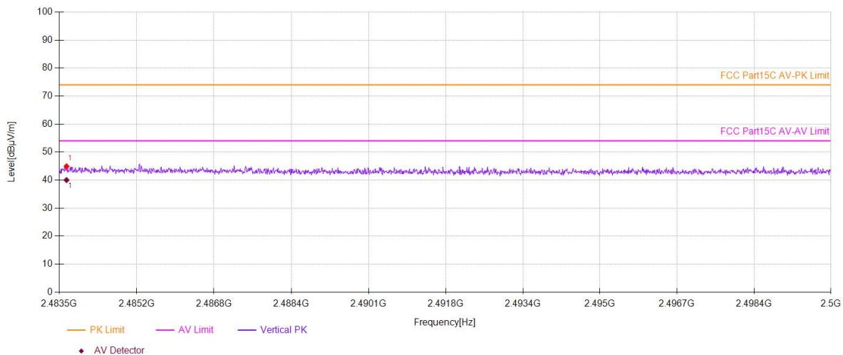
**Note:** (1) All Readings are Peak Value (VBW=3MHz) and Average Value (VBW=10Hz).
