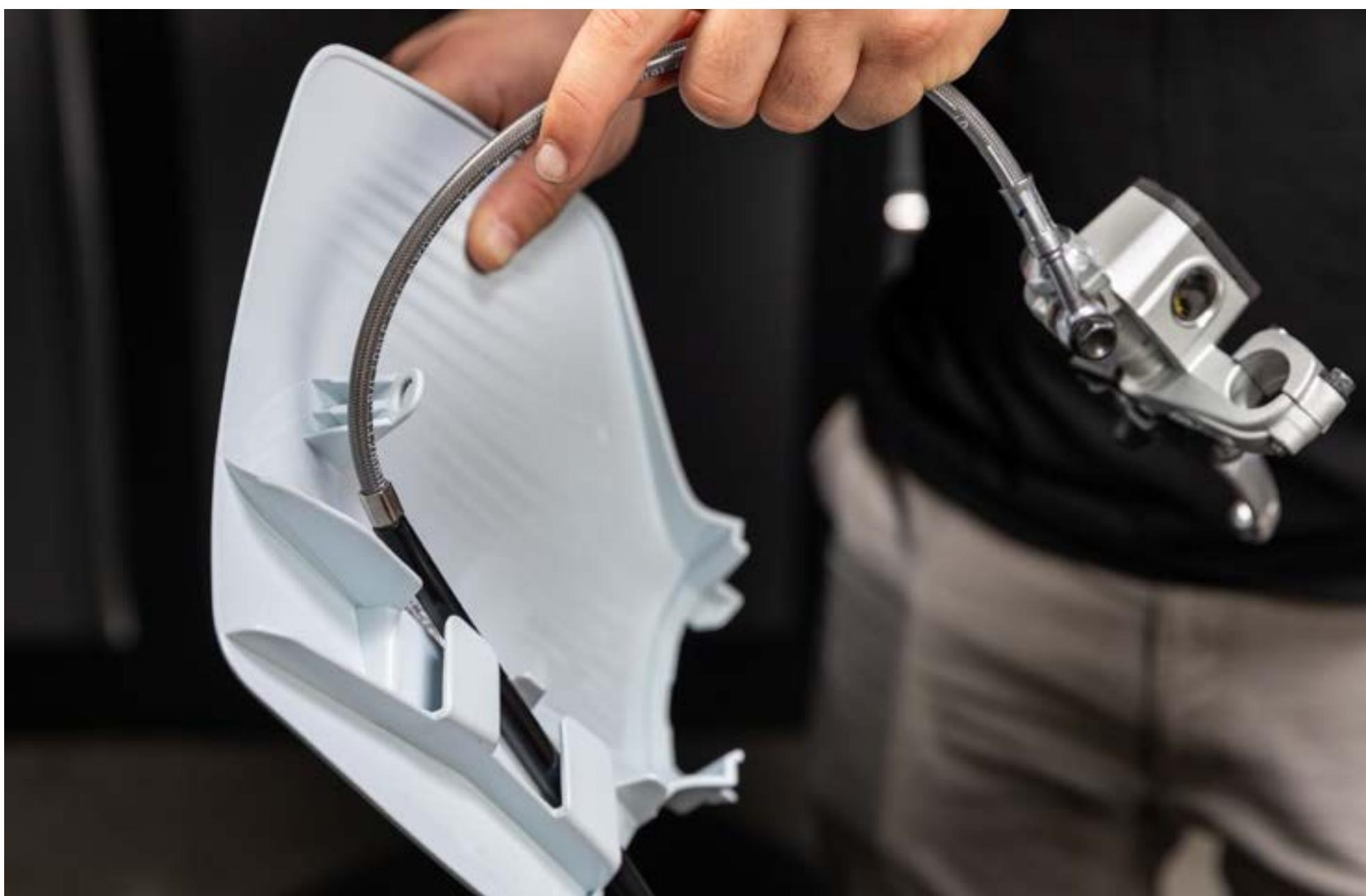
**6** Unscrew the four bolts inside the **docking station** and take it off the **handlebar clamps**.
