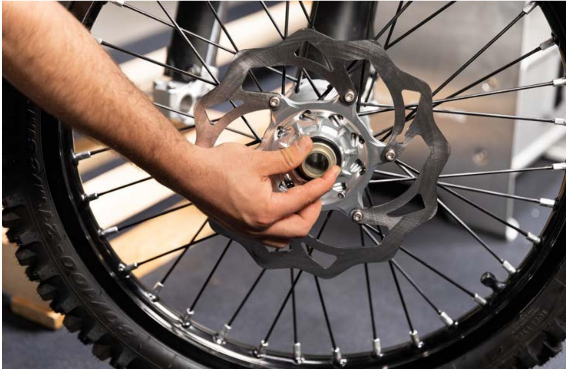
**25** Place the **front wheel** with the **spacers** in between the **fork protectors** and align the **shaft**.
