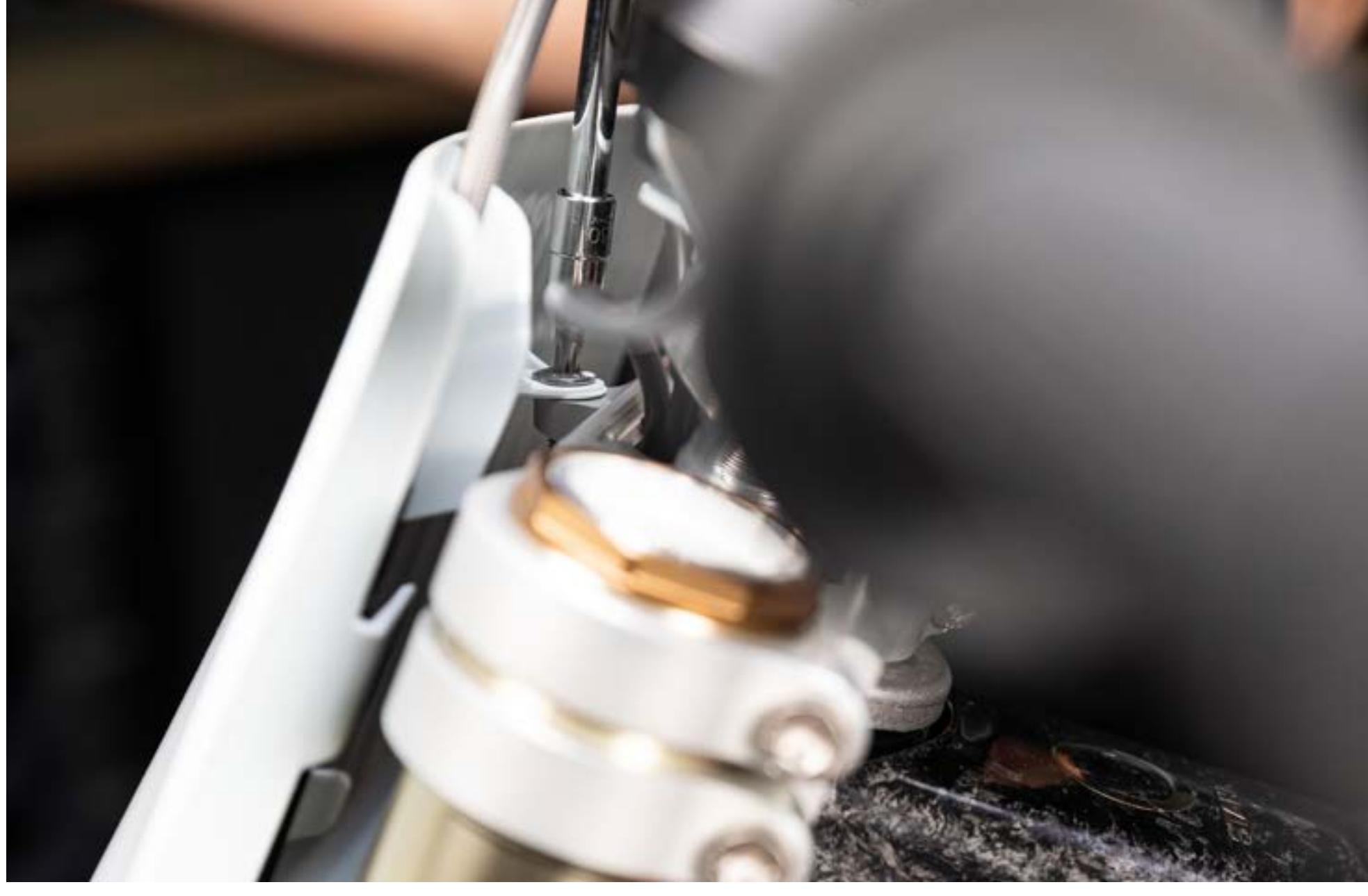
**36** Loosen the **foot peg spindle** on the left side of the motorcycle and take it out.
