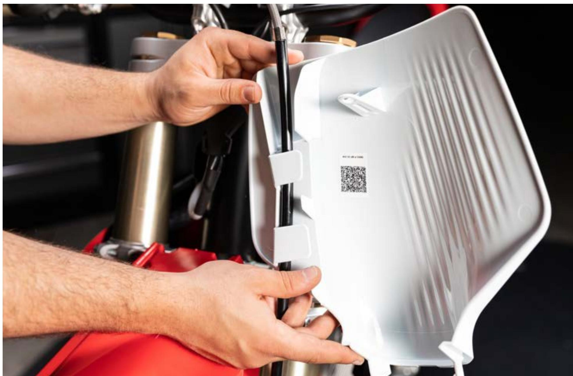
**35** Screw the **number plate** to the triple clamp.
