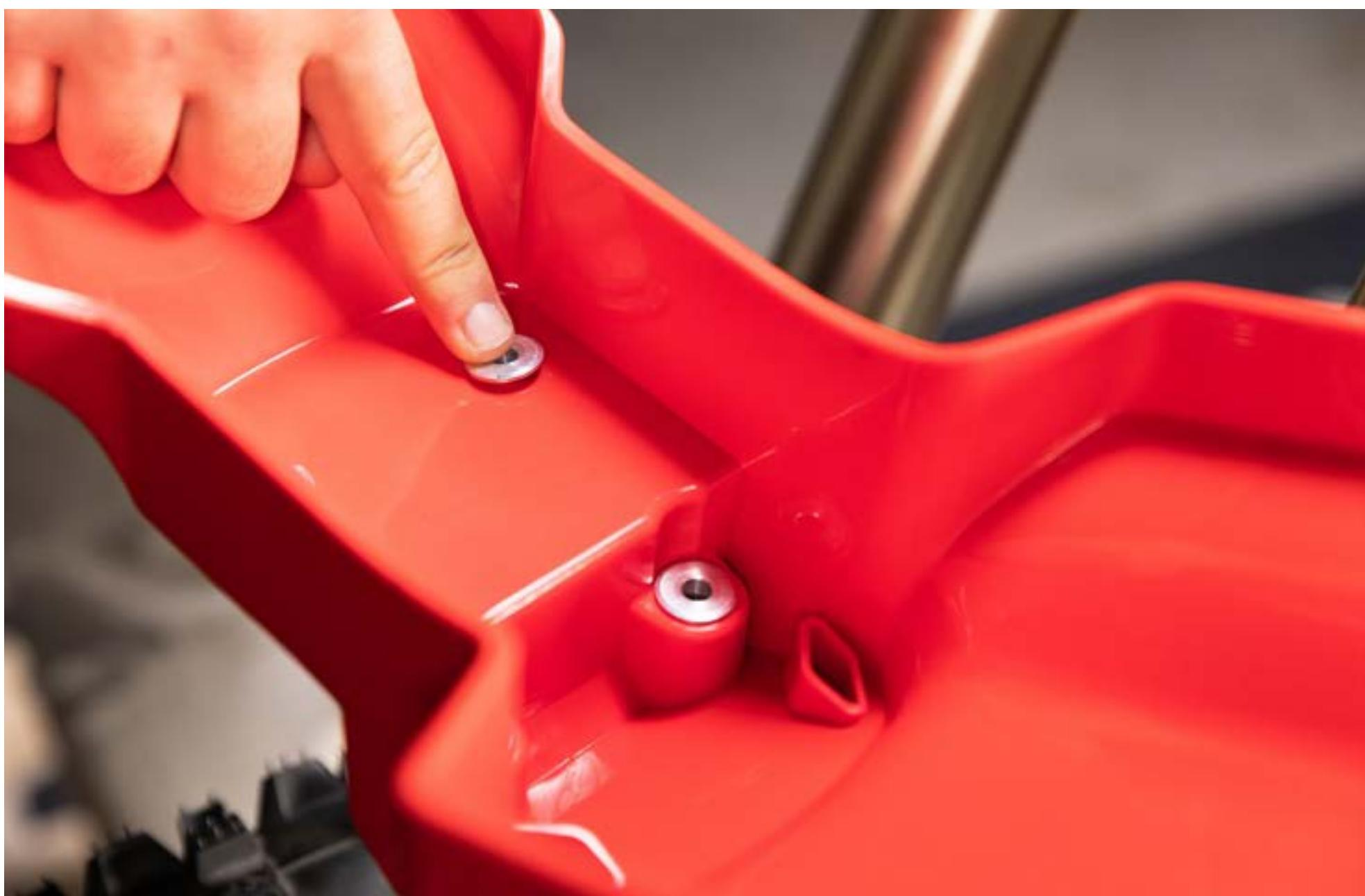
**32** Place the **front fender** in between the fork and align the notches in the **front fender** with the fastening points in the **frame**.
