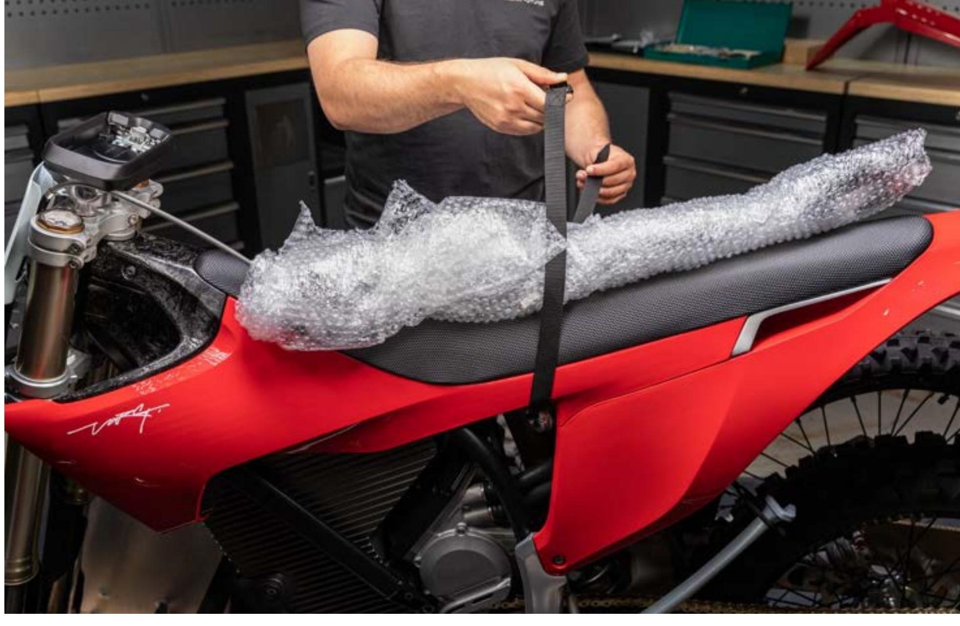
8 Place the **handlebar** on the **handlebar clamps** with the **throttle** on the right side of the motorcycle. Place the **docking station** on top.
