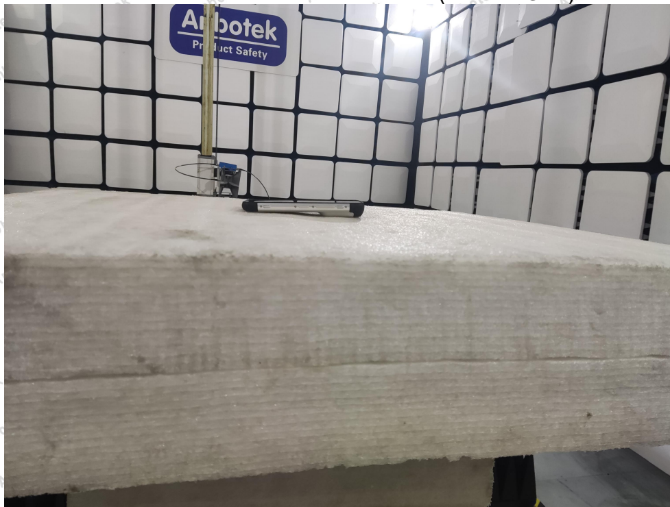
Photo of Radiation Emission Test (above 1GHz)
