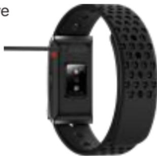
Simply place your device on the magnetic USB charger and plug it into an outlet or USB 2.0+ port to start charging. The red light will stay on while charging, and the green light will appear when fully charged.
